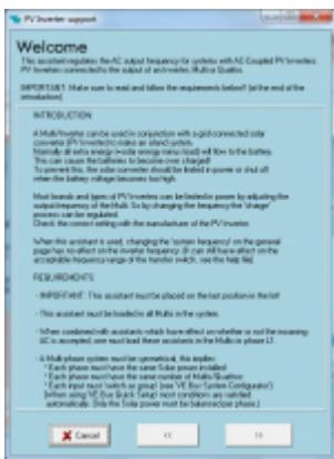
Use this Assistant in Off-grid systems that have AC-Coupled solar power: a grid-tie PV inverter connected to the AC out of a Multi or Quattro inverter/charger.
