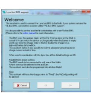
Required in combination with a [Lynx Ion BMS](#), used with our [24 V 180 Ah Lithium system](#). This Assistant can also be used to control the Multi with a third party Lithium system including BMS. See our PDF [Connecting other lithium battery systems to Multis and Quattros](#) for more information.
