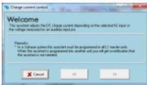
Sets the charge current to a predefined setpoint, based on the active AC Input (for Quattros) or the state of an aux input.
