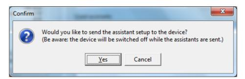
The Inverter/charger will switch off while sending the assistant set up to the Unit. This screen will appear.
