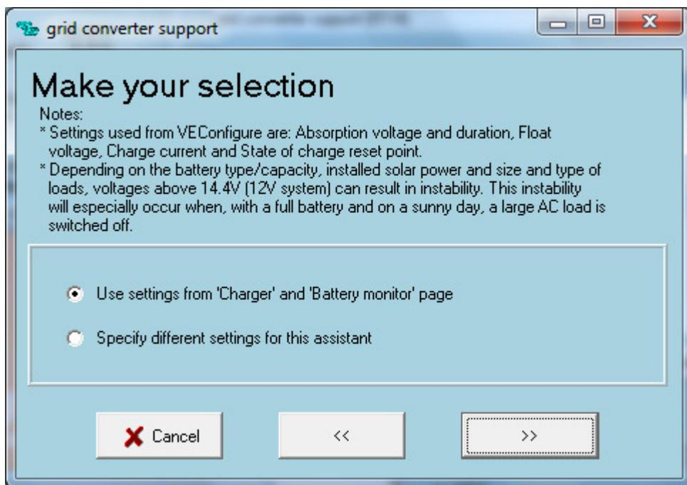
The Restart voltage should not be changed unless it is absolutely necessary. It can be set lower maybe but we don't recommend settings it any higher.
