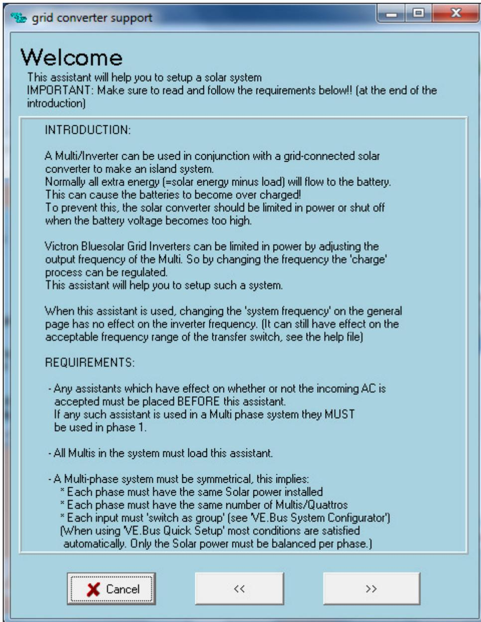
Make sure you know the frequency at which the Grid Inverter will switch off, it must be entered on this page
