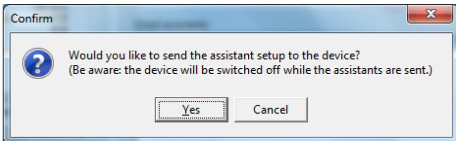
The Inverter/charger will switch off while sending the assistant set up to the Unit. This screen will appear.
