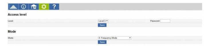
Go to Frequency-Modus and define Frequency start value 50.1Hz and the Frequency end value 51Hz.
