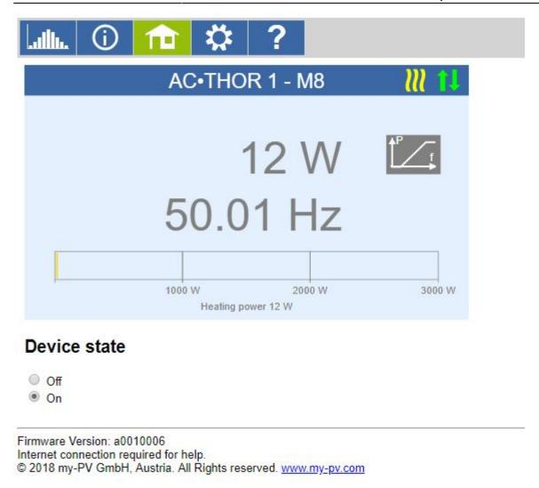
Please check the firmware version on AC-Thor device, must be at least a0010006. Go to setting and select the "Mode". For ESS select "Hot water 3KW", for off-grid systems, select "Frequency-Mode".
