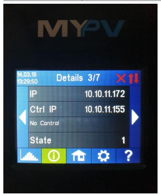
Open a browser, put that IP address into the address field and press enter
