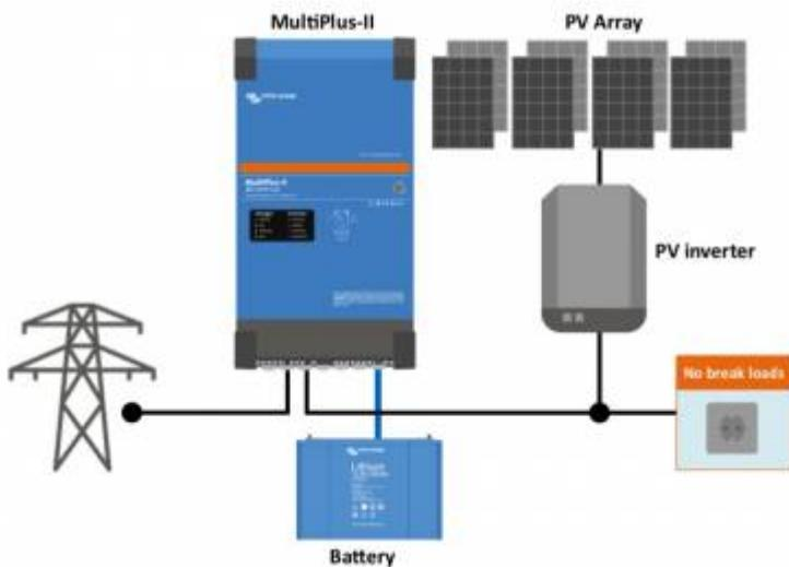
In an AC-coupled system, a grid-tied PV inverter is connected to the output of a Multi, Inverter or Quattro. PV power is first used to power the loads, then to charge the battery, and any excess PV power can be fed back to the grid.
