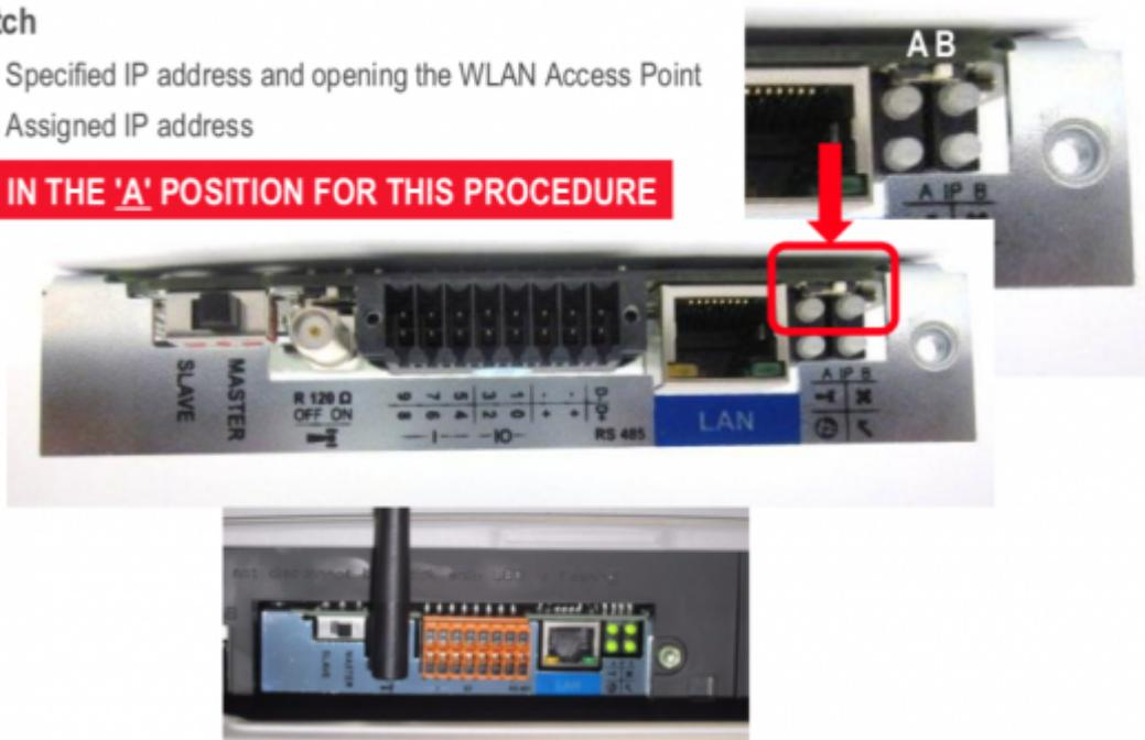
2. Connect both, the Fronius and the GX Device, on the same LAN network, either directly with a LAN cable or using a network switch.
