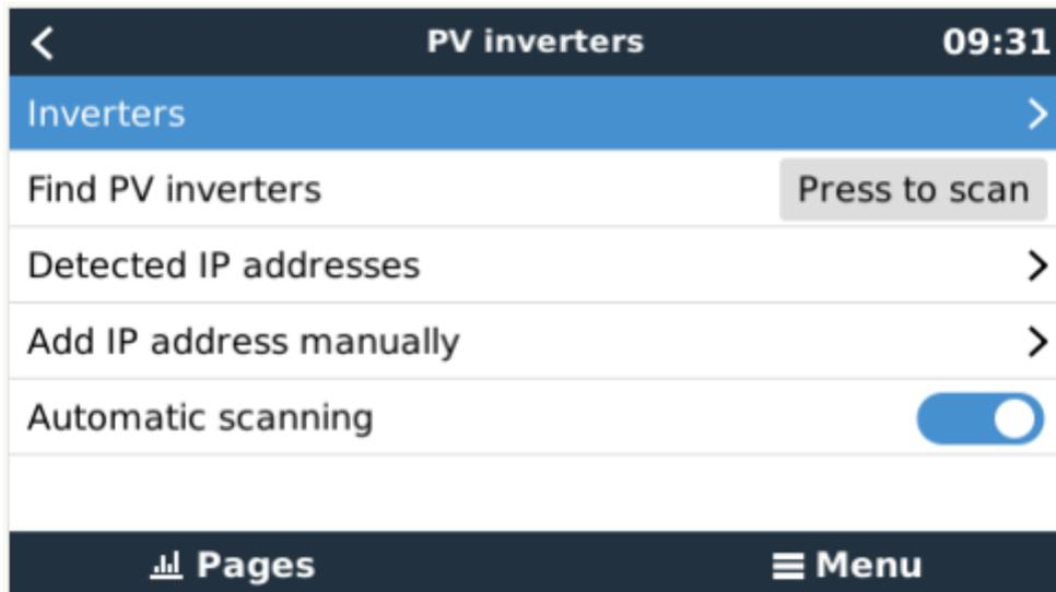
2. Select *Scan* in the GX Device menu, and after completion go into the Inverters submenu to see the results. If scanning does not find the inverter, manually add the IP address of the Fronius Datamanager from its card, or box.
