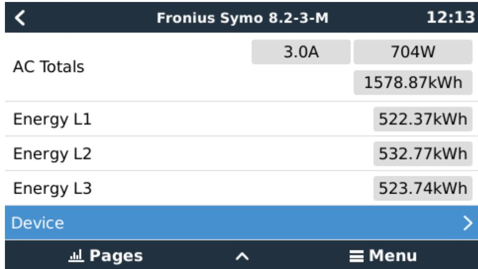
For more details on each device navigate to the Device menu. Here you will find: IP address, Product name, product ID, and Serial number, etc.
