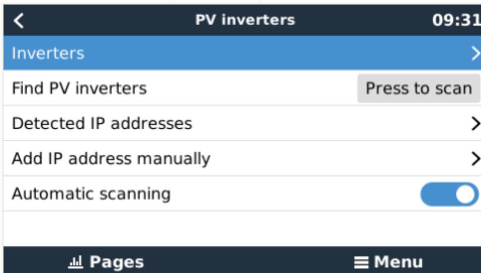
2. Select *Scan* in the GX Device menu, and after completion go into the Inverters submenu to see the results. If scanning does not find the inverter, manually add the IP address of the Fronius Datamanager from its card, or box.
