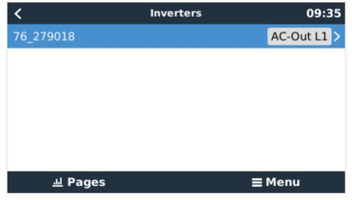
5. Configure the *position* relative to the Multi or Quattro (is it: AC Input / AC Output); and the *show* setting for each inverter in the list:
