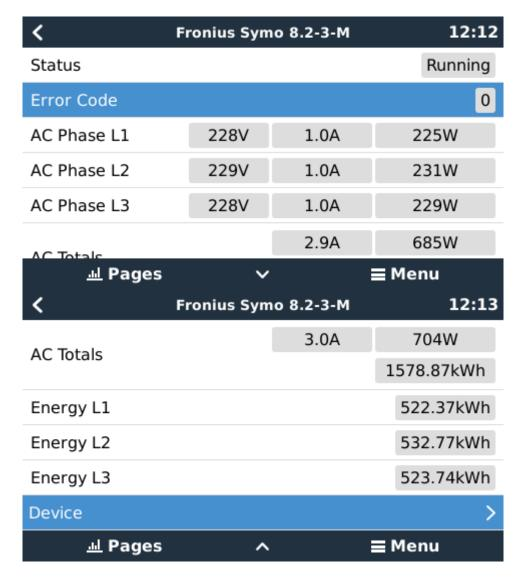
For more details on each device navigate to the Device menu. Here you will find: IP address, Product name, product ID, and Serial number, etc.
