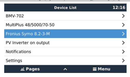
To see the device details, navigate to the menu. Here you can see the current state, current power generated, total power generated.
