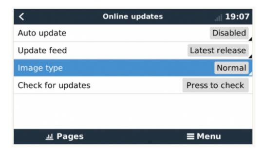
Now, change the Image type to Large. Then go one menu up, and Check for a new version and install that.
